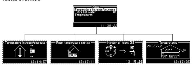
The menu display is only shown in combination with an extra sensor or in a specific operating mode.
